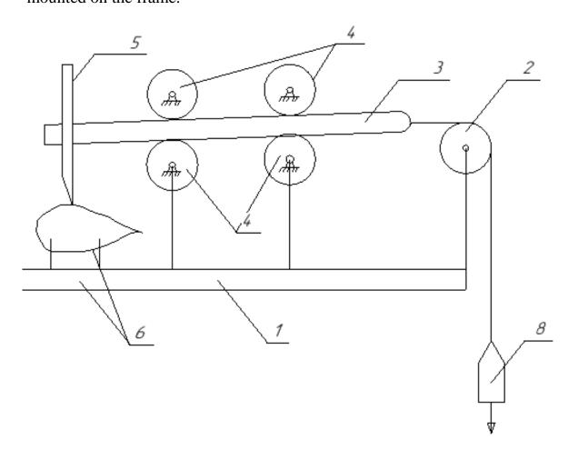
Figure 1. Diagram of a device for determining the force required to separate soil from root crops.
